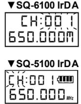
3. Press **SET / MENU** buttons to change the channel number. The corresponding frequency will change accordingly.
