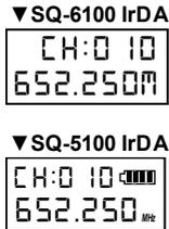
4. 3 seconds after selecting a channel, it will be automatically saved.
